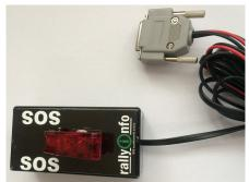
Recommended is a place on floor between seats or on the rooftop of the cabin. In case of usage (emergency assistance required) the crew will switch over the trigger protected by red plastic cover into another position. The GPS unit will send over a SOS signal to central control room of rally HQ. SOS signal can be switched off by placing the cover to normal position.
